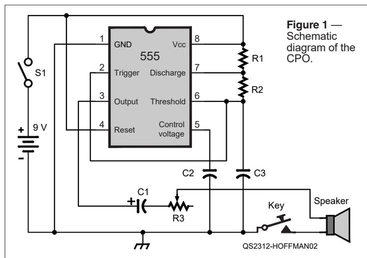
Figure 1 — Schematic diagram of the CPO.
